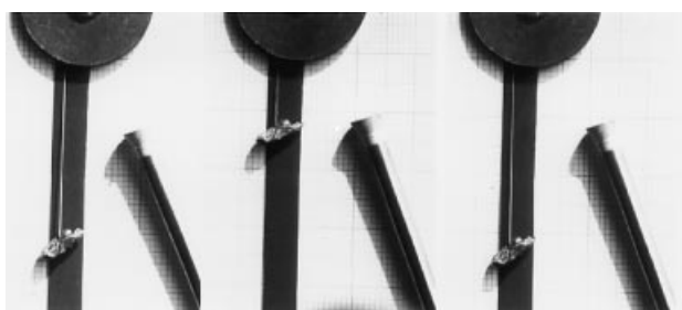
Fig. 5. UV crosslinked fibre of P(12) : (a) at room temperature; (b) heated up to about 150°C; and (c) cooled at room temperature (scaled background smaller subdivision length is 1 mm).
